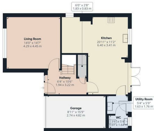
Ground Floor Building 1
